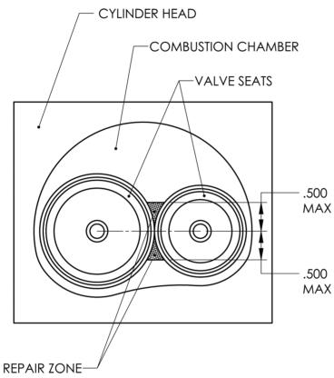
Figure 2 Aluminum Cylinder Head Repair Zone
