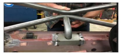
2. All other classes—There is no limit on cage attachment points. The roll cage shall be integrated into the frame or chassis.
