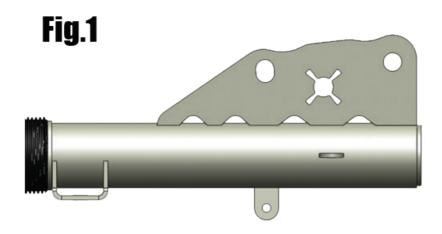
Figure 2: SMG Strut Housing with Camber Slug Installed.
