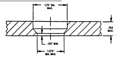
Required Restrictor Plate for GT Engines over 6.0 Liters (366CID).
