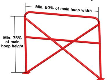
b. Cars must incorporate a main hoop horizontal brace at the approximate level of the driver's shoulders but not lower than the shoulder belt mounting point as described in section 9.3. Driver's Restraint Systems. If a double-diagonal "X" brace is used in the plane of the main hoop, a half-width horizontal brace may be used behind the driver's seat to mount the seat back and shoulder harness as shown in figure 13.
